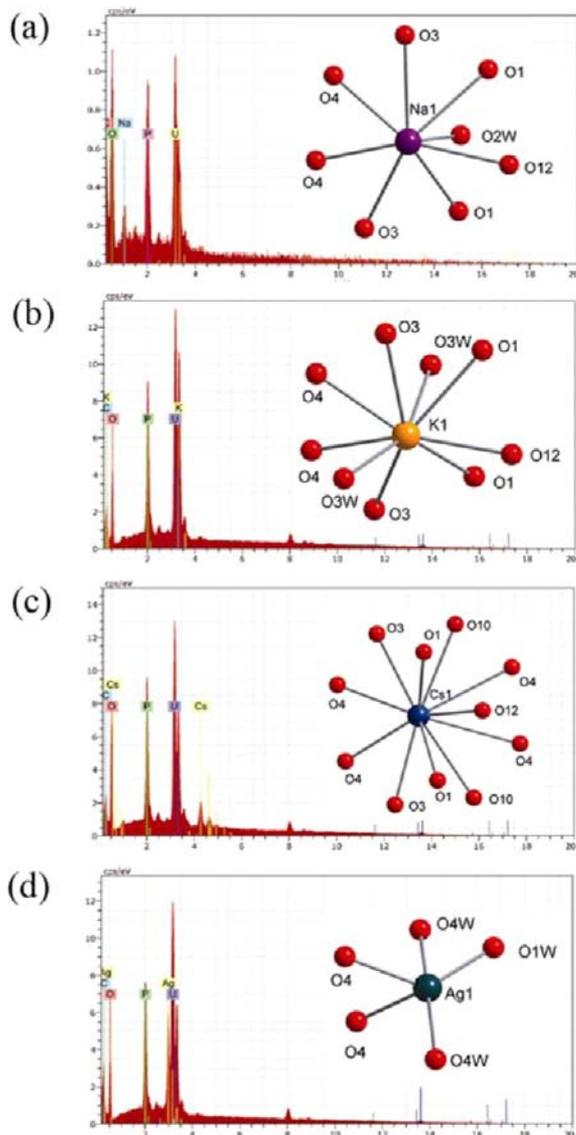
**Figure 7.** EDX results and the coordinated environments of the  $Na^+$  (a),  $K^+$  (b),  $Cs^+$  (c), and  $Ag^+$  (d) cations in the **UP-6** framework (after ion exchange) showing the interactions with the framework oxygen atoms and water molecules.
