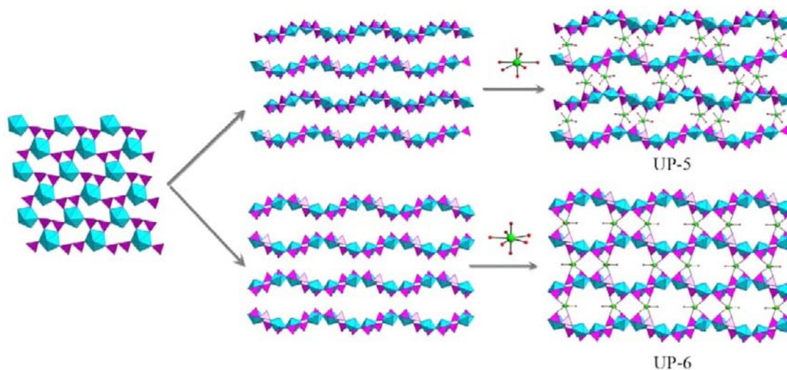
**Figure 6.** Layers are stacked in A,  $-A$  sequence and further connected by three-connected  $UO_7$  pentagonal bipyramids to form UP-5, and by four-connected  $UO_7$  pentagonal bipyramids to form UP-6, respectively. Color code: blue, U; purple, P; red, O; green, the linkage uranium atoms.
