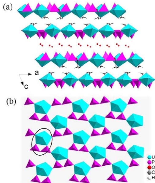
**Figure 3.** (a) Layers are stacked in a sequence of A,  $-A$  in UP-4, (b) the single layer and its SBU in highlight.
