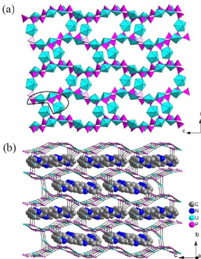
**Figure 4.** (a) Polyhedral view along the *a* axis of UP-5 showing the elliptic channels and its SBU in highlight, (b) bipy molecules exist in the channels of UP-5.
